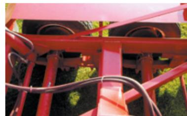
*The 16K PLUS features heavy duty running gear connected to the frame with a leaf spring suspension. The dual axles can be equipped with optional Hydraulic Brakes.*
