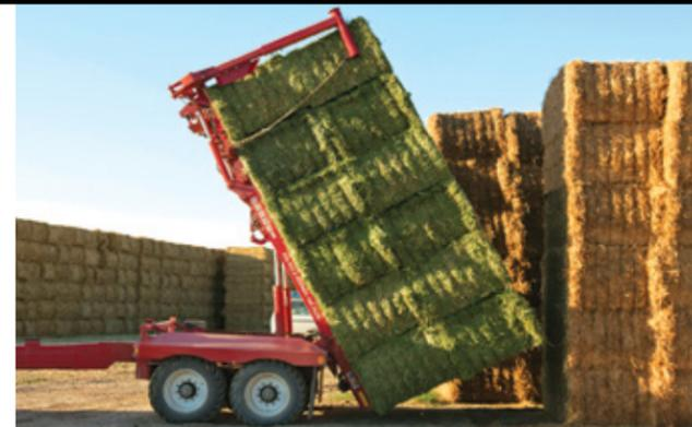
*Once the bed is vertical, the alignment arms are opened, and the Bale Runner is driven forward to remove the forks from under the stack.*
