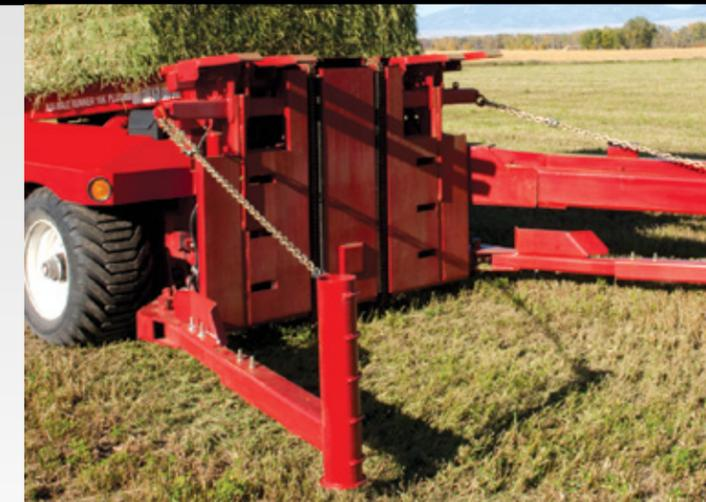
Bales are easily picked in any orientation. The alignment arms center the first bale - grab hooks hold the bale in place - the loader lifts slightly off the ground so the bale DOESN'T DRAG while traveling to the second bale. Stair stepping the bales during
