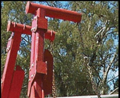
Optional Short Bale Bracket attachments can be mounted on the alignment arms to pick up shorter wet silage bales.
