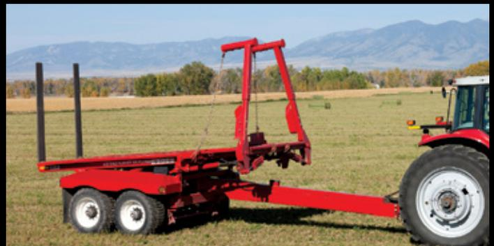
Work Light Kit Option: Two 7" LED (adjustable) work lights securely mounted to the front of the hitch for optimal lighting when picking bales at night. Assists with seeing, turning, and picking bales, as well as backing up and unloading the bales.
