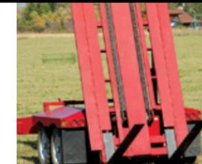
*Strong and sturdy forks hold the bales in place while stacking and unloading.*
