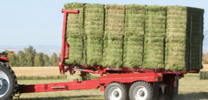
Computer controlled to maximize speed and to simplify your bale handling operation - to pick up and load bales, the operator toggles only the loader button. The computer determines the motion of the alignment arms, loader, grab hooks and power slider. It's that simple. A six button joystick controls the motion of the bed, hitch and pushoff.
