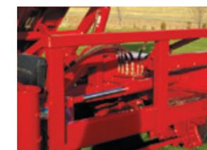
*The hitch cylinder is cushioned at both ends to prevent shock and is reinforced with a thick plate top and bottom at the main stress points.*
