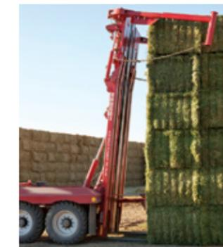
*Steering with the hitch allows the operator to easily see and line up to the existing stack.*
