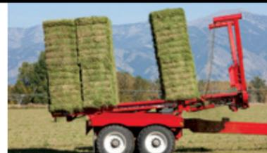
*A power slider on the 16K PLUS pushes each row of bales back automatically and is reset by the computer once the bales are all the way back.*
