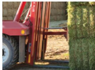
*The 16K PLUS features a pushoff that when activated assists in moving the bales off the forks as you drive away.*
