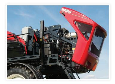
Engine and hydraulic service checkpoints are easy to access from the walkway by the engine compartment.
